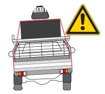
Vehicle performance is affected by tall/heavy loads on racks, especially sideways.
