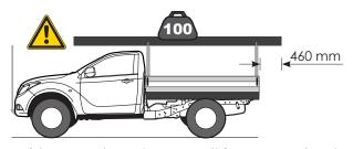
Avoid unequal overhangs as this may overload the front support and/or flex over the cab.
