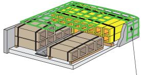
Loose items must be under cargo nets and must not extend more than 100 mm above the sides. Tie down larger items with restraints.
