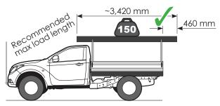
Max 450 mm rear overhang. Max 150 kg for evenly spread load.
