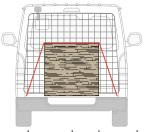
Secure heavy loads centrally across the vehicle with rubber or timber under the load.
